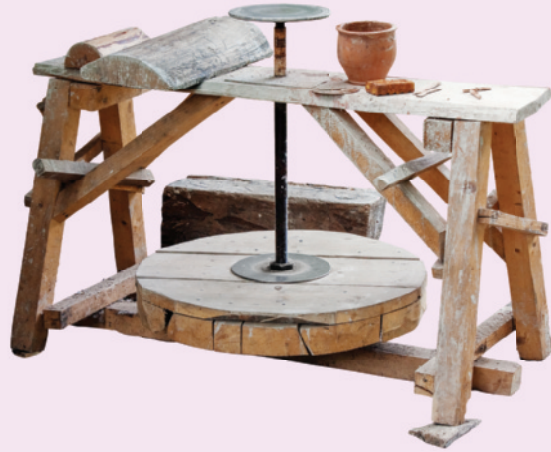
■ Figure 14.6 A flywheel on a potter's wheel
