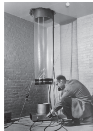
■ Figure 13.52 Rebka at work in the basement of the Jefferson laboratory at Harvard; the polythene tube contains helium to focus the gamma photons into a narrow beam
