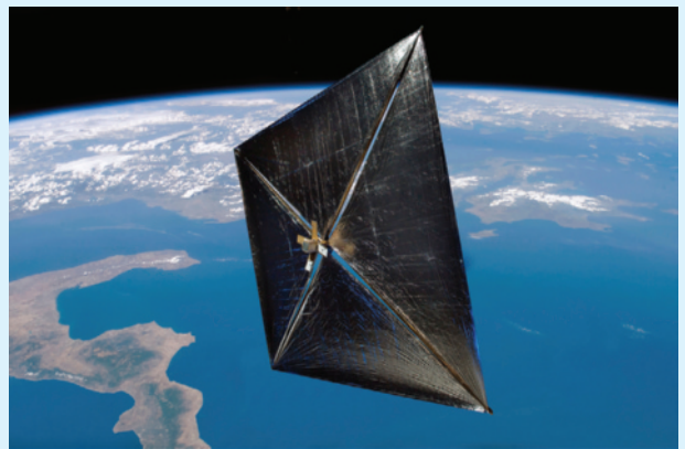
■ Figure 13.39 A solar sail is an enormous reflector that uses the solar wind as a propulsion mechanism. Although the total force exerted by the solar radiation is small, over a long period of time it is sufficient to propel space probes to high velocities
