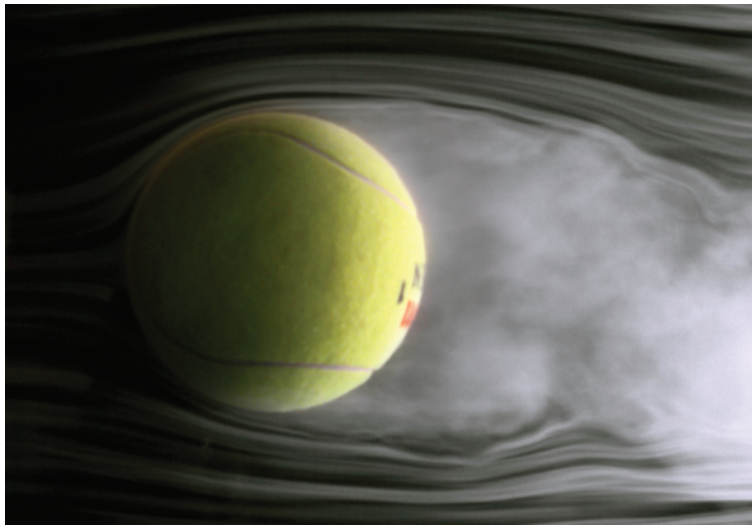
■ Figure 14.56 Streamlines around a tennis ball in a wind tunnel
