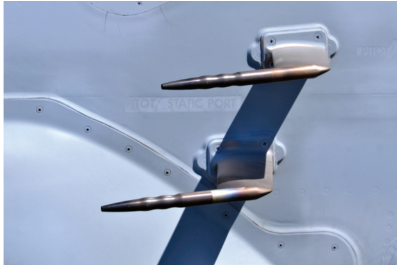
■ Figure 14.60 Pitot tubes on an aircraft
