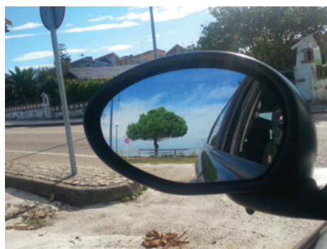
■ Figure 15.25 Wide field of vision produced by a car's wing mirror
