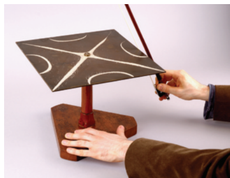
■ Figure 14.73 Demonstrating the vibrations of a metal plate
